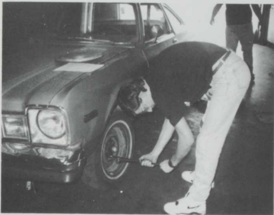
Ron Malone takes the wheel off the shop car to do an inspection on the brakes.
